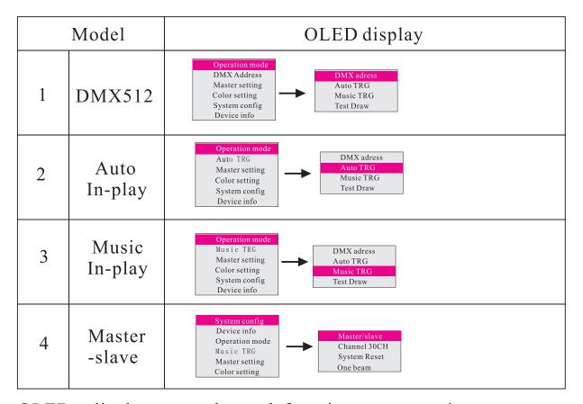
OLED display control panel function menu setting, as following::
