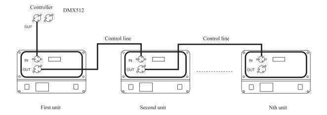
Caution: Please remember the signal output of last machine must connect the attached circle plug .The circle plug connect a 120 resistor between 2 feet and 3 feet canon plug. The signal reflects phenomena can be avoided by using circle plug during DMX 512 signal transfer. (DMX TERMIN ATOR CONNECTION):
