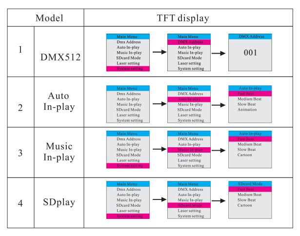
TFT LCD display control panel function menu setting, as following::
